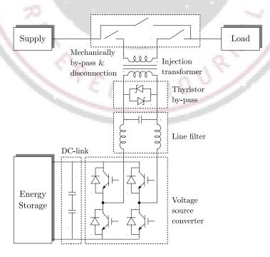
Figure 3: The Basic Elements of a DVR in a Single-Phase Representation
