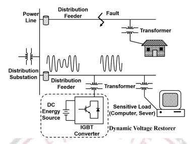
Figure 2: Operating Principle of Dynamic Voltage Restorer
