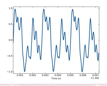
Figure 6: Detection of a Non-Symmetrical Voltage Dip
